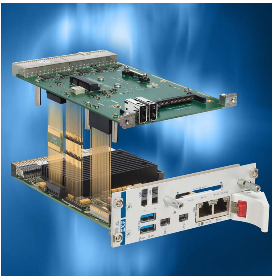
Sample Mezzanine Side Card 8HP Assembly
